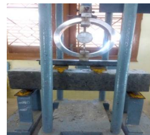
Fig 4.2 Test Set Up for Flexural Strength
