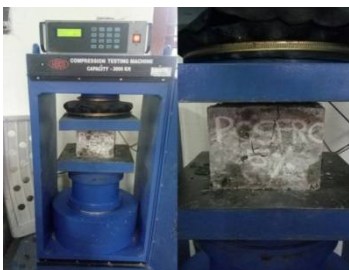
Fig 4.1 Compression test (before and after testing)
