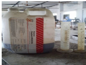
Fig. 2.3 Super plasticizer III. MIX DESIGN
